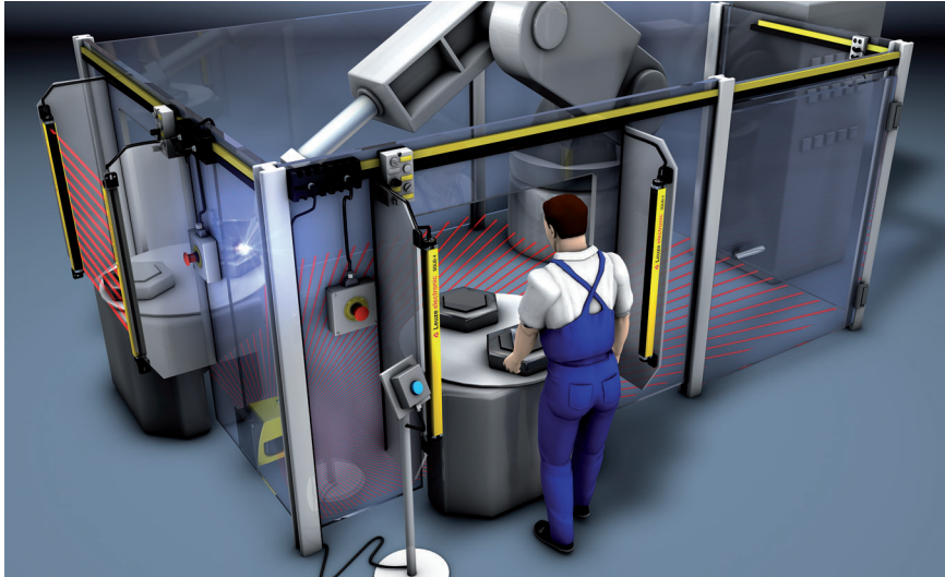
AS-Interface Safety at Work-based robot application with 2 release circuits
