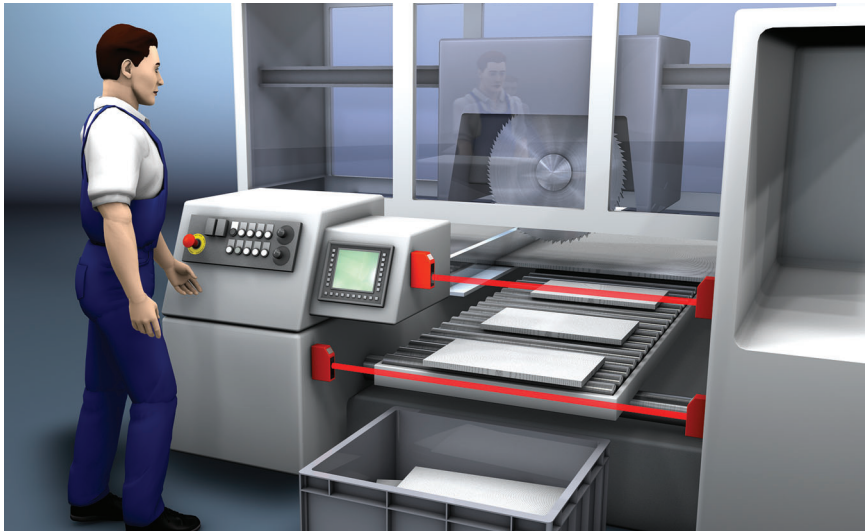
Guarding a wood processing center with SLSR 46B Single Light Beam Safety Devices and MSI-T safety monitoring device
