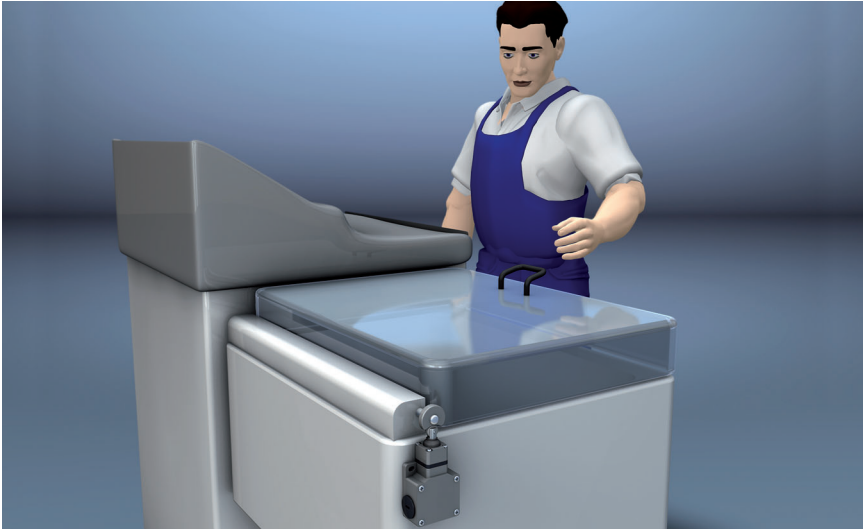
Safety Position Switch on machine with a protective device and swivel joints – a typical application, e.g. in automated parts processing
