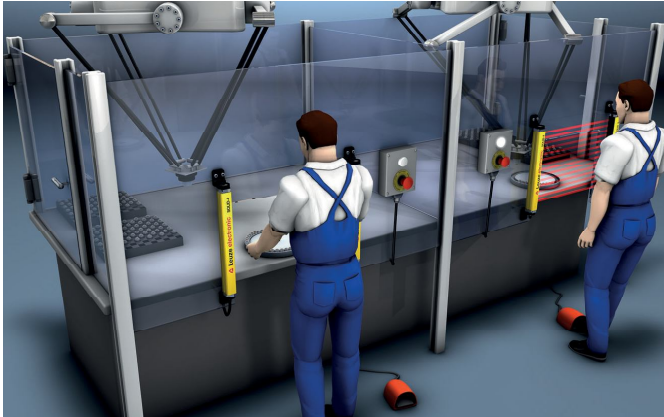
Control of individual safety components with programmable Safety Controllers.
